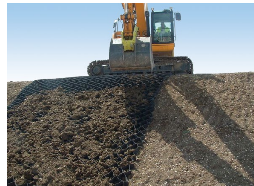
FIGURE 9 TYPAR GeoCell GS cells transfer downward forces laterally, reducing loads on underlying soils to provide stabilization over poor soil conditions, protect soil and roots from compaction, and provide site access for light, heavy, and industrial vehicles. Photo courtesy TYPAR Geosynthetics.
